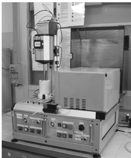
Fig. 4 Flow reactor combining ultrasound and microwaves.
